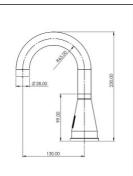
Non-contact self-closing DN 15 Washtable-tap, stainless steel satin; with rotating and lockable curved spout, aerator\*, optosensor.
